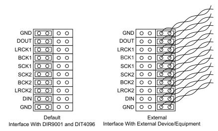
Figure 2. Flexible PCM Audio Interface
