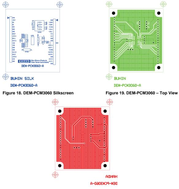
Figure 20. DEM-PCM3060 - Bottom View
