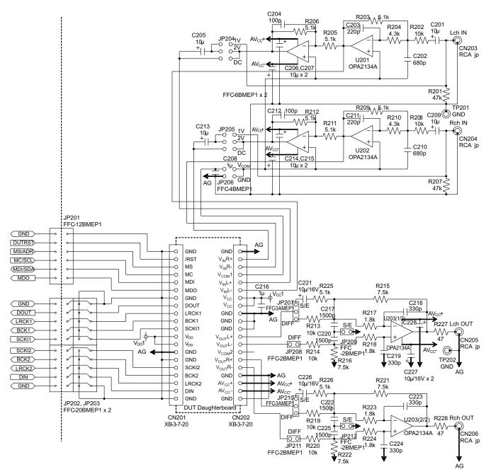
Figure 13. LPF and Buffer for Analog Input/Output
