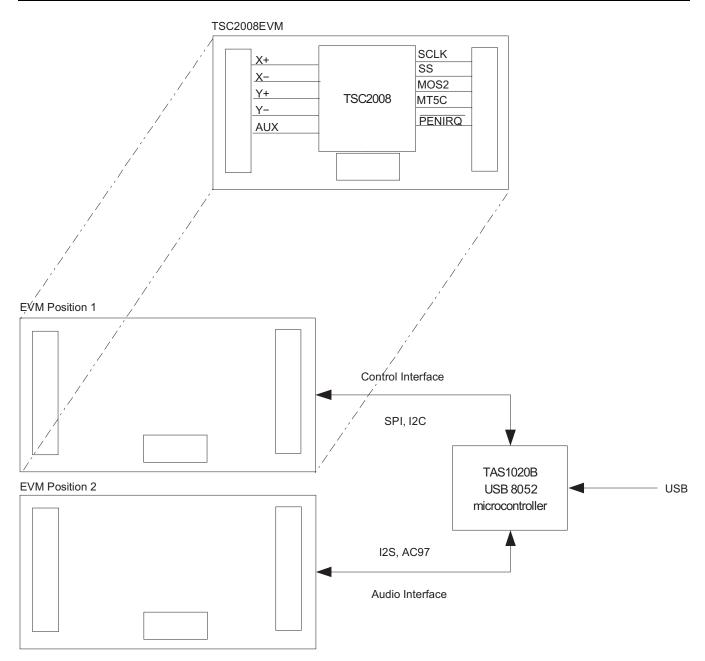
Figure 1. TSC2008EVM-PDK Block Diagram
