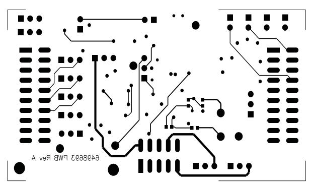
Figure 6. Layer 4 (Bottom Signal Plane)
