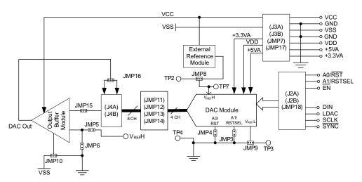
Figure 1. DAC8164/65EVM Block Diagram
