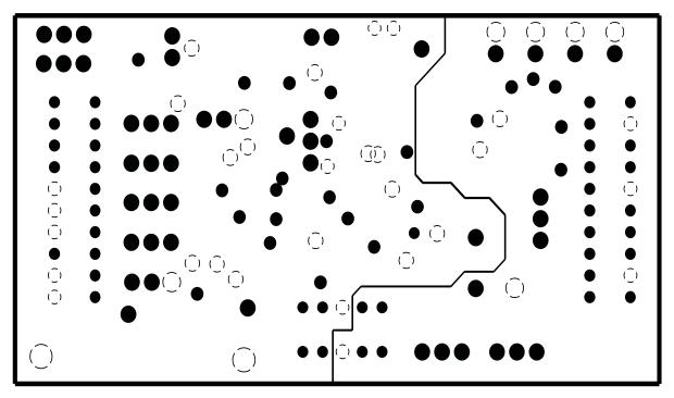
Figure 4. Layer 2 (Ground Plane)
