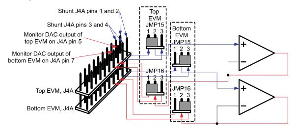
Figure 10. DAC8164/65EVM Output Operational Amplifier Jumper Configuration for Stacking
