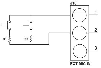
Figure 14. Headset Detection Circuit
