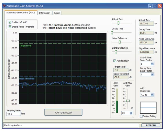
Figure 12. Automatic Gain Control Panel
