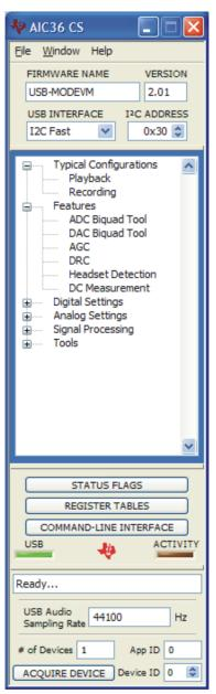
Figure 2. Initial Screen of TLV320AIC36EVM-K Software
