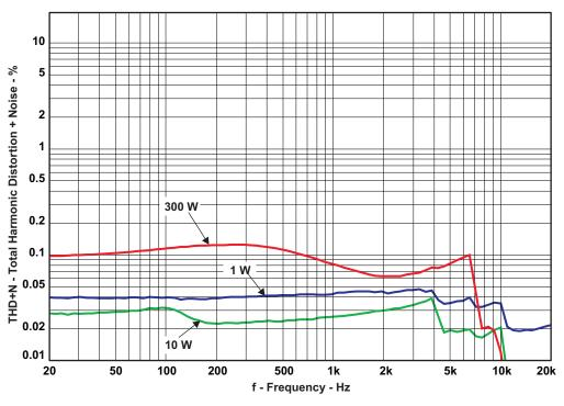
Figure 9. THD+N vs Frequency (PBTL  $-2 \Omega$ )
