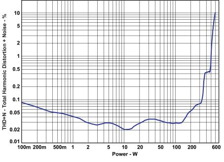
Figure 6. THD+N vs Power (PBTL –2  $\Omega$ )
