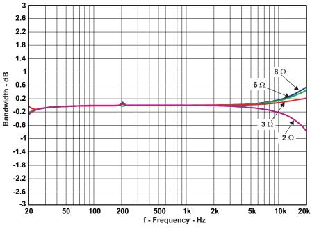
Figure 16. Frequency Response (PBTL)
