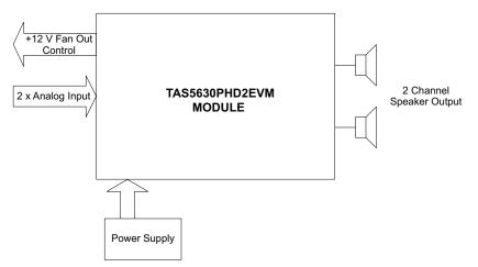
Figure 1. Integrated PurePath<sup>™</sup> Premier Pro Amplifier System
