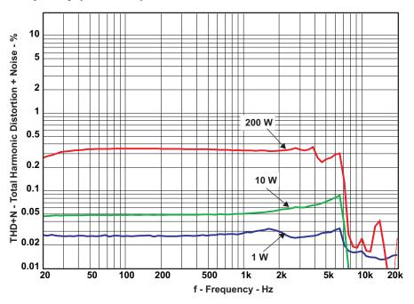
Figure 7. THD+N vs Frequency (BTL –4 Ω)
