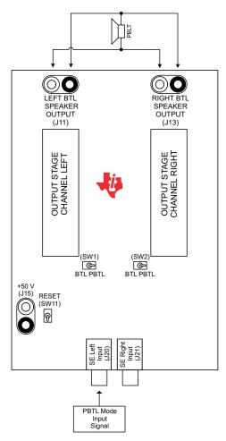
Figure 3. Figure 3. PBTL Mode Configuration
