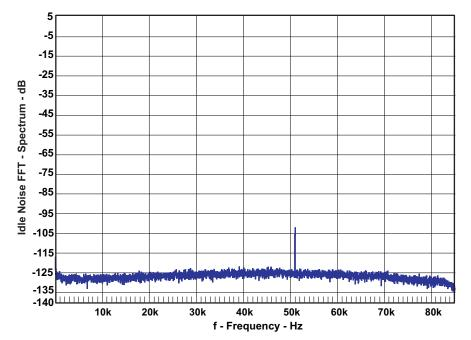
Spurious tone at 52 kHz has it's origin from the TL2575 switching voltage regulator.
