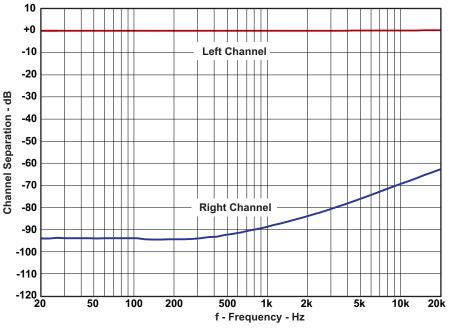
Figure 14. Channel Separation
