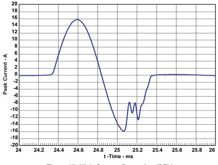
Figure 17. High-Current Protection (BTL)
