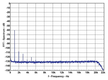
Figure 10. FFT Spectrum with -60-dBFS Tone (BTL)
