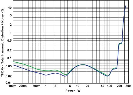
Figure 4. THD+N vs Power (BTL – 4  $\Omega$ )
