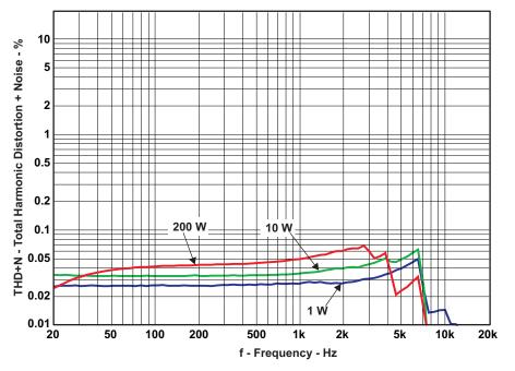
Figure 8. THD+N vs Frequency (BTL –8 Ω)
