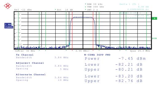
Figure 9. WCDMA ACPR (DAC Ch. B): DAC Clk = 614.4 MHz, 2x Int, 30-MHz Offset
