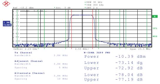
Figure 8. WCDMA ACPR: LO = 1966.4 MHz, DAC Clk = 614.4 MHz, 2× Interpolation, f<sub>s</sub>/4 mixing, 30-MHz Offset
