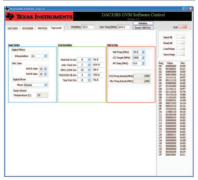
Figure 2. DAC3283 GUI Front Panel
