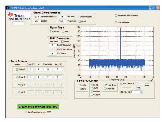
Figure 4. TSW3100 MultiTonePattern Programming GUI
