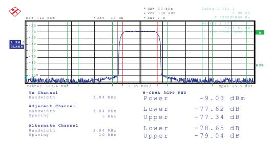
Figure 10. WCDMA ACPR (DAC Ch. B): DAC Clk = 614.4 MHz, 2× Int, f<sub>s</sub>/4 Mixing, 30-MHz Offset; 183.6-MHz IF
