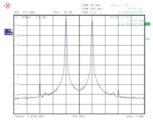
Figure 6. Two-Tone IMD Performance: LO = 2400 MHz, DAC Clk = 614.4 MHz, 2x Interpolation, IF = 20, 21 MHz
