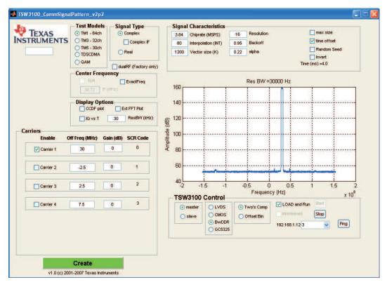
Figure 5. TSW3100 CommsSignalPattern (WCDMA) Programming GUI
