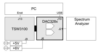
Figure 3. Test Setup Block Diagram
