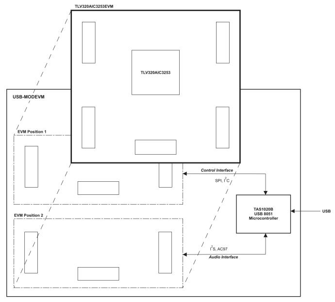
Figure 1. TLV320AIC3253EVM-K Block Diagram
