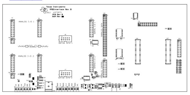
Figure 19. MMB Interface Board
