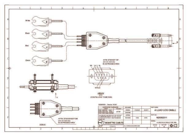
Figure 48. ECG Cable Drawing
