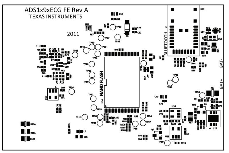
Figure 50. Bottom Layer Placement
