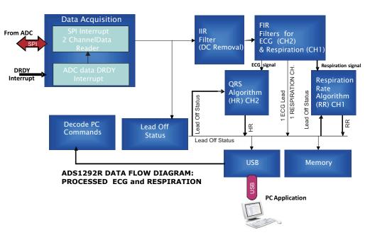
Figure 37. Live Data Stream Mode Data Flow for ADS1292R
