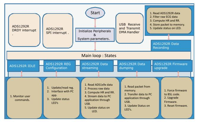
Figure 35. Firmware Architecture
