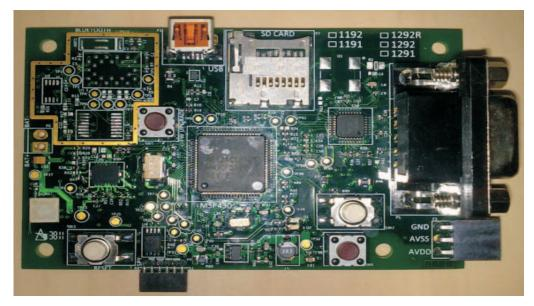
Figure 1. ADS1x9xECG-FE Demonstration Kit
