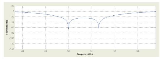
Figure 40. Frequency Response for the MBF Filter (50Hz Notch)
