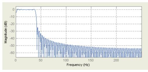
Figure 42. Frequency Response for the Band Pass Filter
