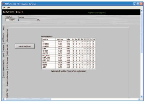
Figure 24. Register Configuration – Register Map
