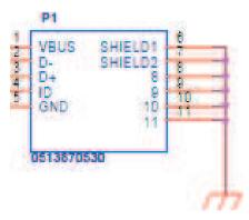
Figure 47. USB Mini Connector Pin Outs
