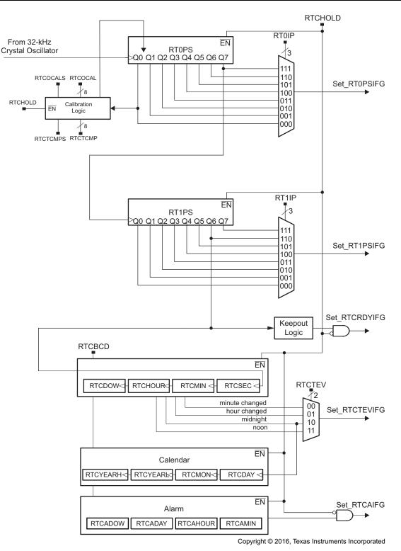
Figure 1-1. RTC\_C Block Diagram (RTCMODE = 1)
