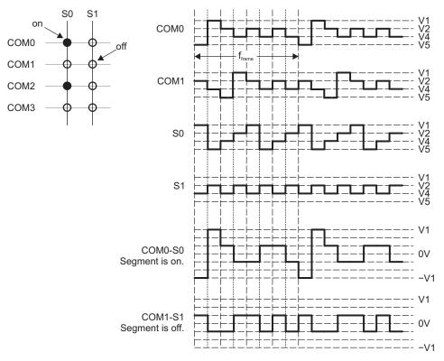
Figure 1-8. Example 4-Mux Waveforms
