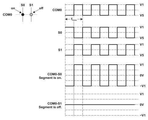
Figure 1-5. Example Static Waveforms
