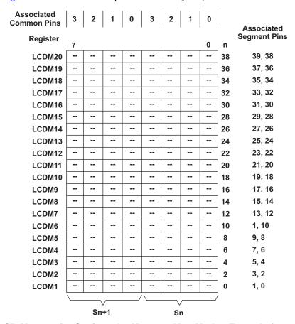
Figure 1-2. LCD Memory for Static and 2-Mux to 4-Mux Mode - Example for 160 Segments
