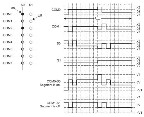
Figure 1-11. Example 8-Mux, 1/3 Bias Low-Power Waveforms (LCDLP = 1)
