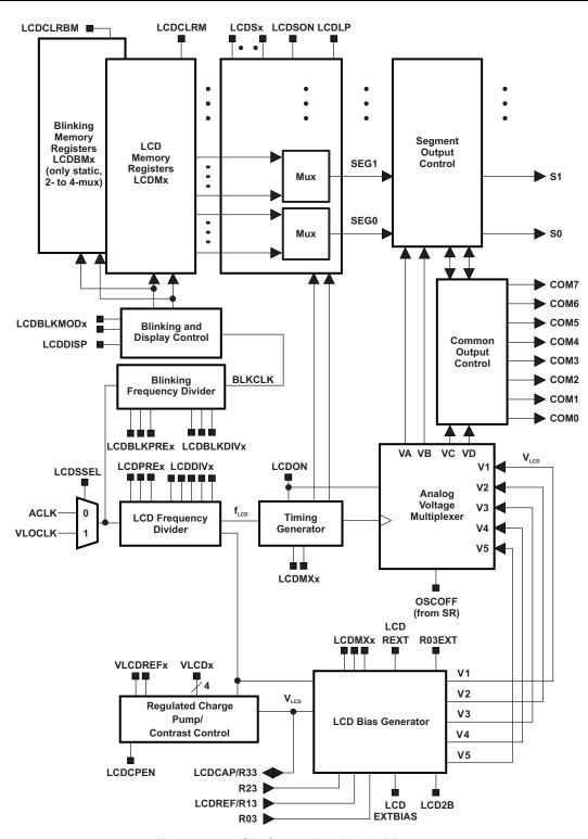
Figure 1-1. LCD Controller Block Diagram
