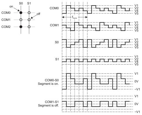
Figure 1-7. Example 3-Mux Waveforms
