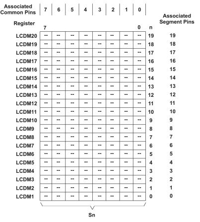
Figure 1-3. LCD Memory for 5-Mux to 8-Mux Mode - Example for 160 Segments
