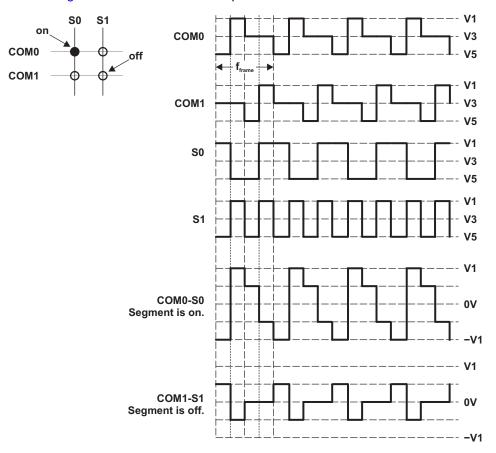
Figure 1-6. Example 2-Mux Waveforms
