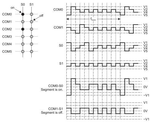
Figure 1-9. Example 6-Mux Waveforms
