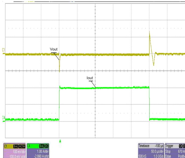
NOTE: C4 - Load Current Step (100mA - 2.A), C1 VOUT - Output voltage transient response.
