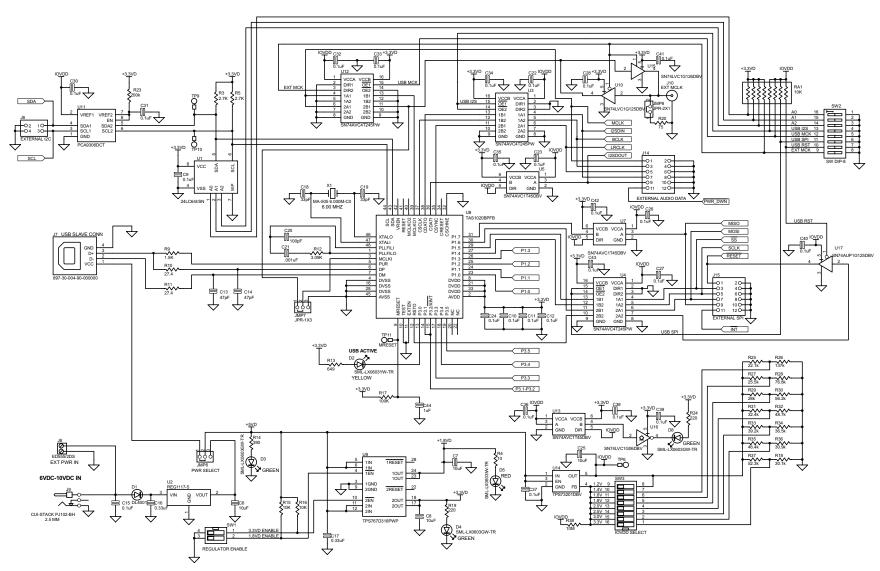
Figure 21. USB-MODEVM Schematic (Sheet 2 of 3)
