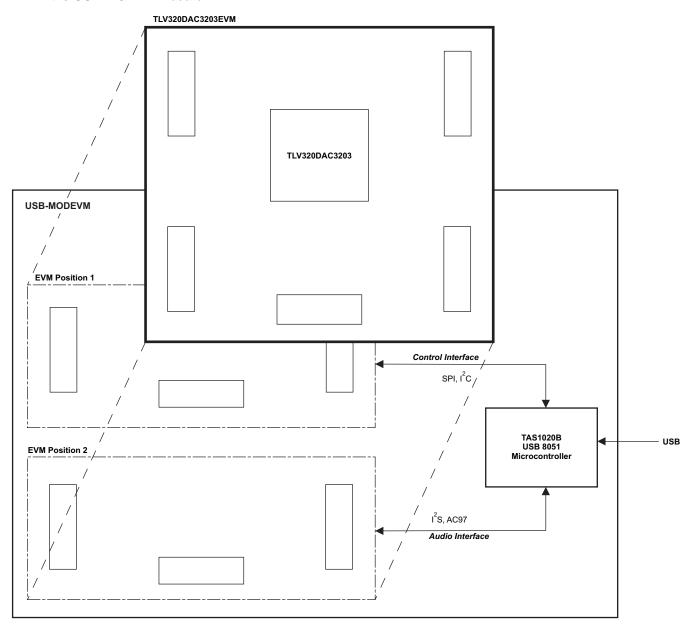
Figure 1. TLV320DAC3203EVM-K Block Diagram
