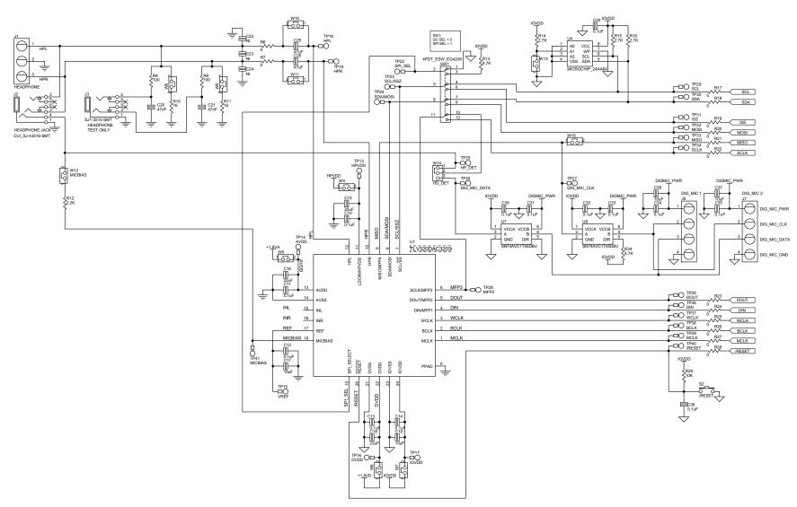
Figure 10. TLV320AIC3253EVM Schematic (Sheet 1 of 2)
