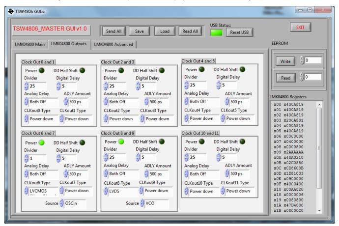
Figure 3. LMK04800 Output Tab
