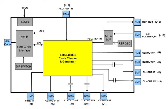
Figure 1. TSW4806EVM Block Diagram
