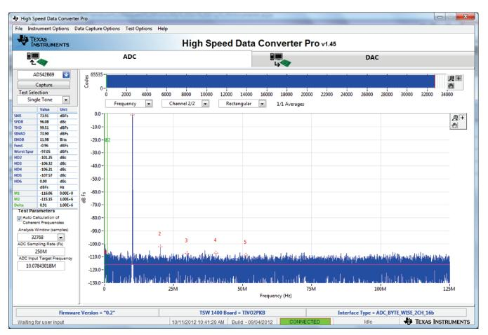
Figure 6. ADS42LB69 Sample Capture using the TSW1400
