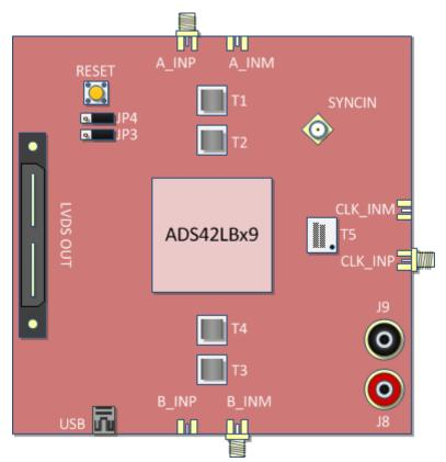
Figure 1. Block Diagram of the ADS42LBx9EVM
