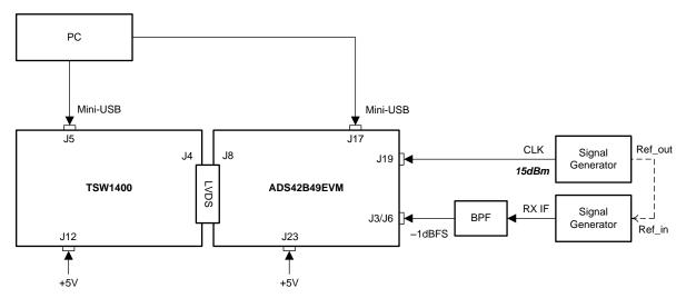
Figure 3. Test Set-Up Block Diagram
