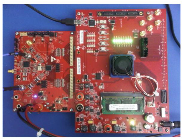
Figure 2. ADS42B4xEVM and TSW1400
