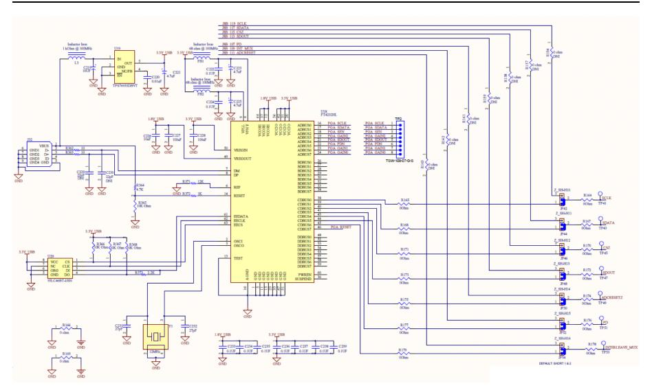
Figure 76. PGA5807 Schematic, (Sh. 14 of 16), FTDI Serial Interface
