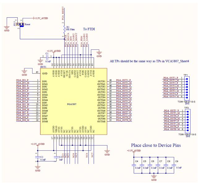
Figure 63. PGA5807 Schematic, (Sh. 1 of 16), PGA5807 Device
