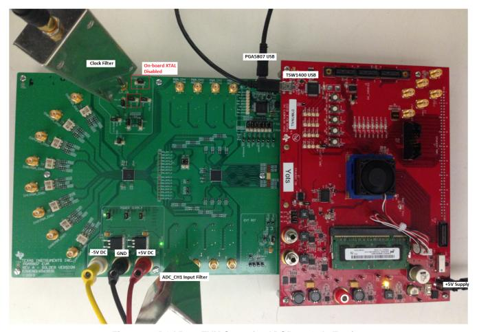
Figure 40. PGA5807 EVM Setup for ADS5296 Only Testing
