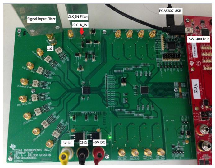
Figure 43. PGA5807 + ADS5296 Gain Test Setup
