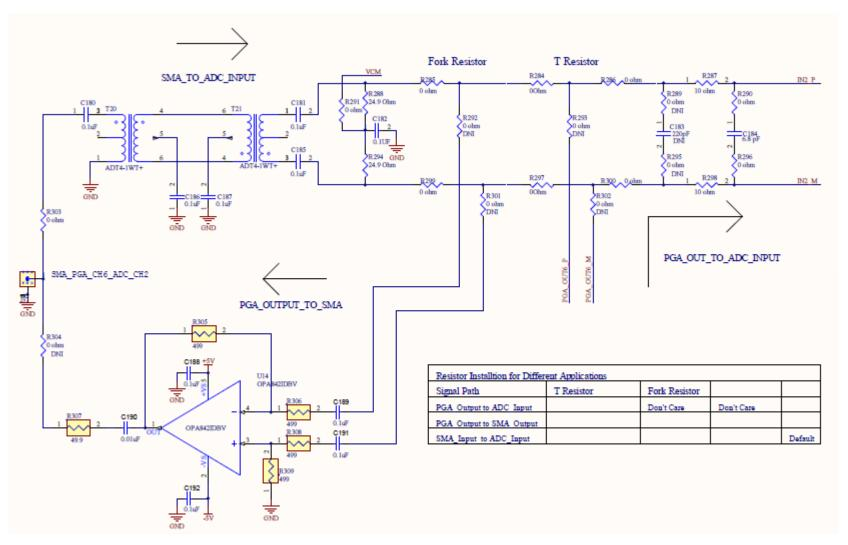
Figure 73. PGA5807 Schematic, (Sh. 11 of 16), PGA\_CH6, ADC\_CH2
