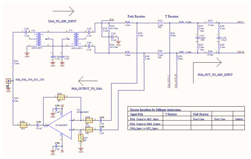
Figure 71. PGA5807 Schematic, (Sh. 9 of 16), PGA\_CH4, ADC\_CH8
