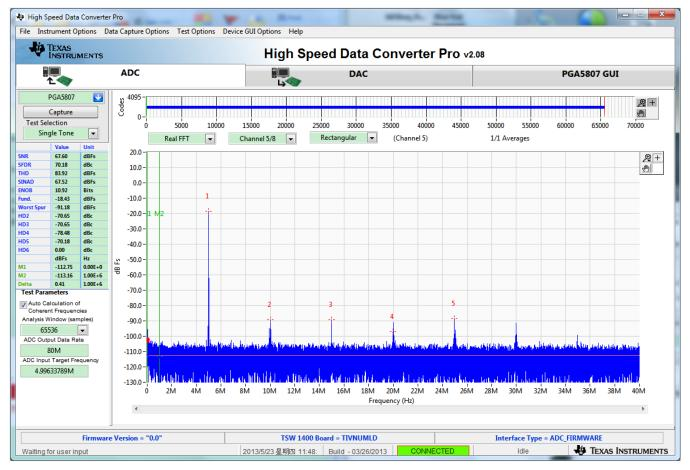
Figure 47. PGA5807+ADS5296 Gain Test Capture 2
