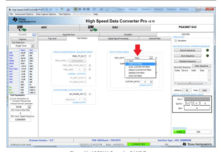
Figure 32. ADS5296 Setup for RAMP Test
