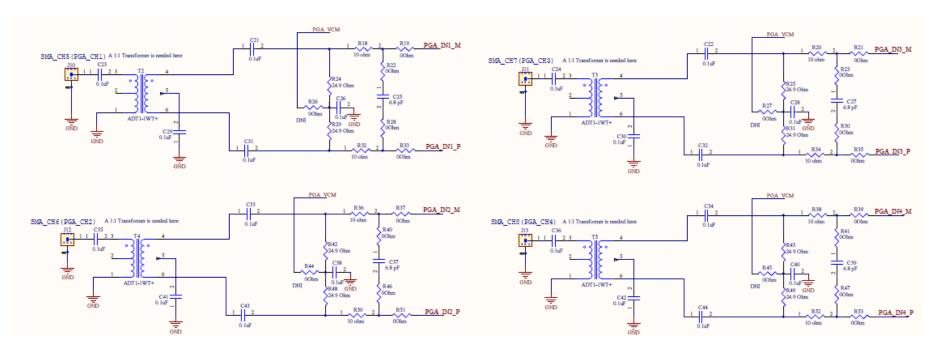
Figure 66. PGA5807 Schematic, (Sh. 4 of 16), PGA5807 Analog Inputs Ch1-4
