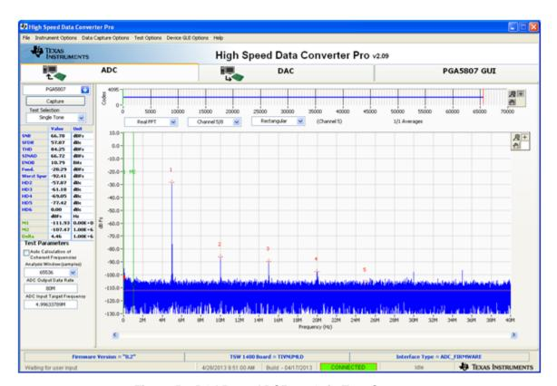
Figure 51. PGA5807+ADS5296 Gain Test Capture 4
