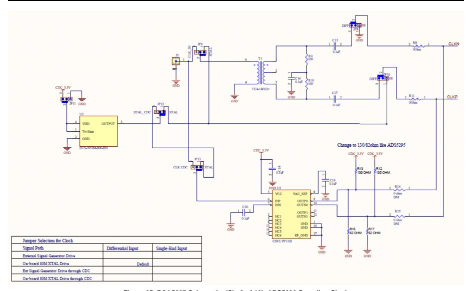
Figure 65. PGA5807 Schematic, (Sh. 3 of 16), ADS5296 Sampling Clock
