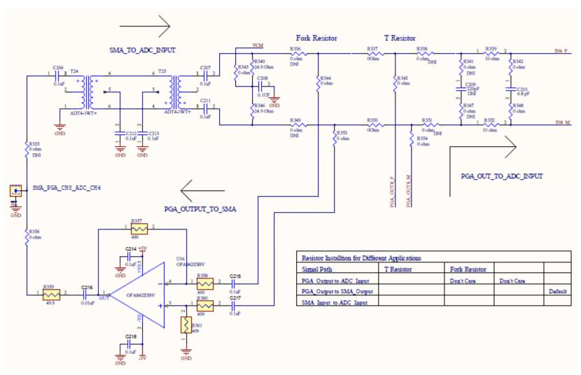
Figure 75. PGA5807 Schematic, (Sh. 13 of 16), PGA\_CH8, ADC\_CH4
