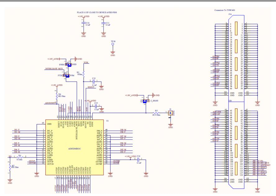
Figure 64. PGA5807 Schematic, (Sh. 2 of 16), ADS5296 Device
