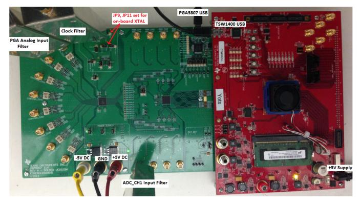
Figure 19. TSW1400 and PGA5807 Sptup
