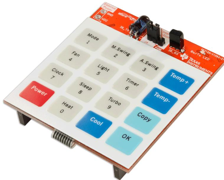
**Figure 1. BOOST-IR BoosterPack**
