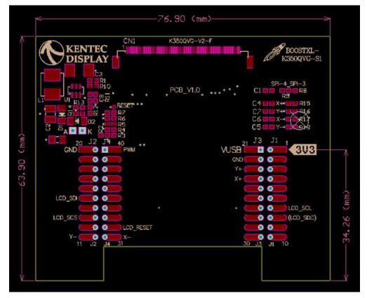
Figure 3. BoosterPack Pinout (View From Bottom of PCB)
