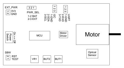
Figure 6. Motor Board Layout
