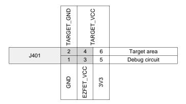
The TARGET\_VCC is sourced from the EZ-FET circuit for energy tracing. To bypass the EZ-FET and power from the USB power circuit directly, connect 1-2 (GND to TARGET\_GND) and 5-6 (3V3 to TARGET\_VCC) of the J401.
