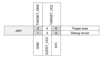
The target area of the board can also be powered by external power by connecting pin 2 (TARGET\_GND) and pin 4 or 6 (TARGET\_VCC) of the J401.
