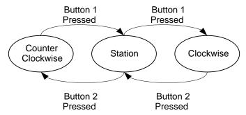
Figure 7. Control Rotating Direction in Manual Mode
