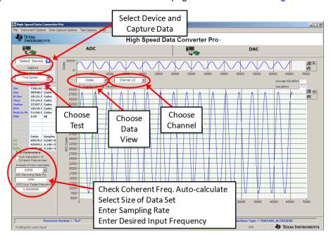
Figure 3. HSDC Pro GUI Main Panel
