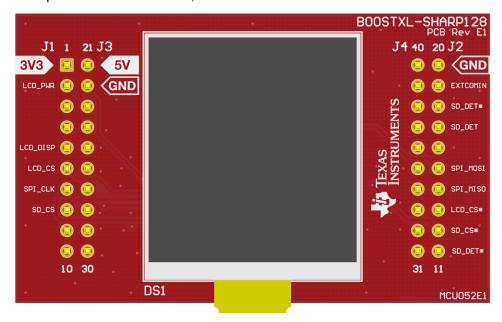
Figure 1. BOOSTXL-SHARP128 BoosterPack™ Plug-In Module
