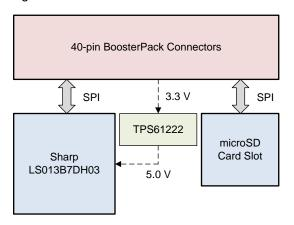
Figure 3. BOOSTXL-SHARP128 Block Diagram
