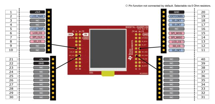
Figure 4. Connector Pinout for LaunchPad Development Kit and BoosterPack Plug-in Module
