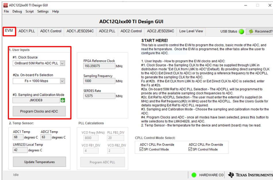
Figure 3-2. Configuration GUI EVM Tab
