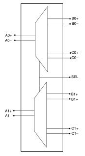
Figure 1. TMUXHS4212 Functional Block Diagram
