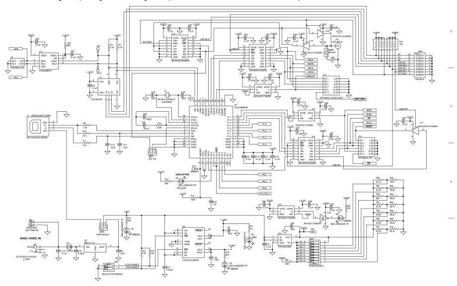
Figure 3-2. USB-MODEVM Schematic
