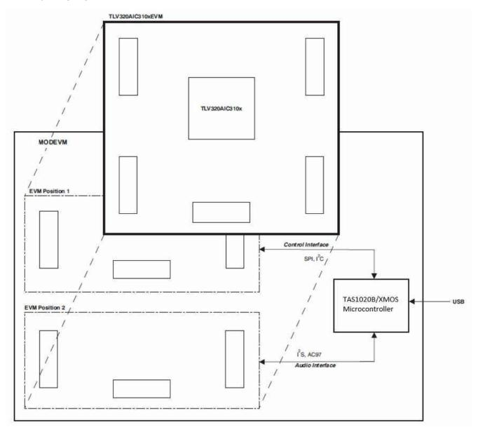
Figure 3-1. TLV320AlC310xEVM-PDK Block Diagram
