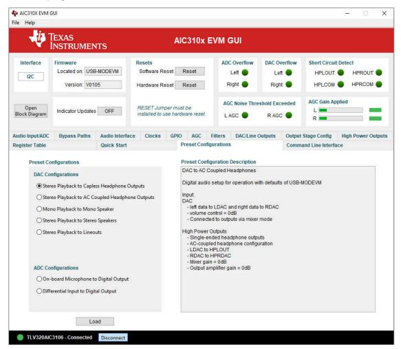
Figure 2-3. Preset Configurations Tab
