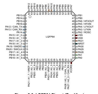
Figure 2-3. LQFP64 Pinout (Top View)
