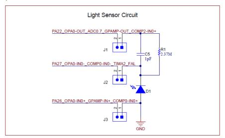
Figure 2-9. Light Sensor Circuit
