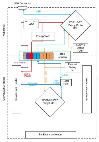
Figure 2-5. Isolation Jumper Block
