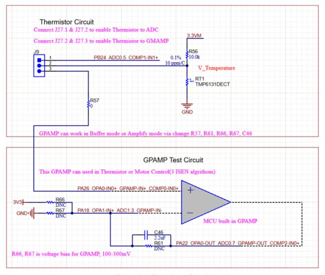
Figure 2-8. Thermistor Circuit
