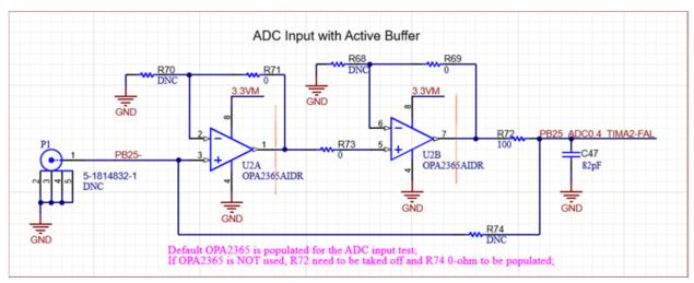
Figure 2-7. External OPA Circuit
