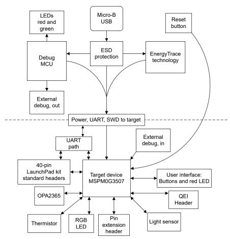
Figure 2-2. Block Diagram
