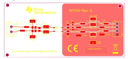
Figure 3-2. ISOM8110DFGEVM PCB Layout - Top
