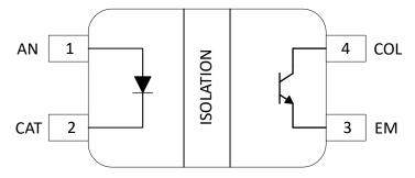
Figure 2-2. ISOM8110 Single-Channel Opto-Emulator with Analog Transistor Output Pin Configuration
