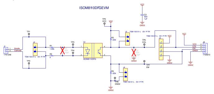
Figure 3-1. ISOM8110DFGEVM Schematic
