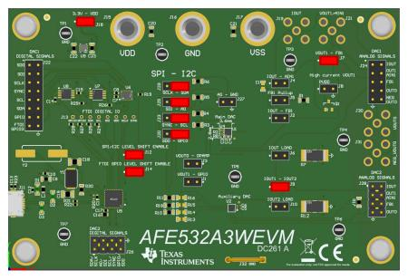
Figure 2-4. AFE532A3WEVM Parallel IOUT Jumper Settings
