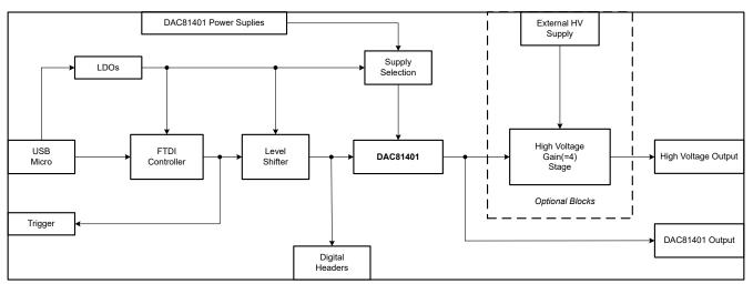
Figure 1-1. DAC81401EVM Functional Block Diagram
