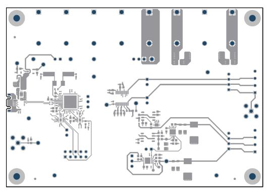
Figure 4-8. DAC81401EVM PCB Bottom Layer Layout
