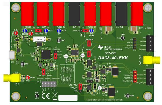
Figure 3-1. Default Header Settings with High Voltage Gain Stage Enabled
