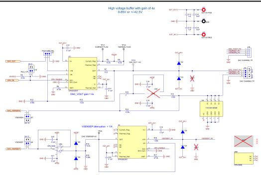
Figure 4-3. DAC81401EVM Schematic : High Voltage Gain Stage
