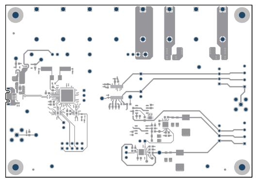
Figure 4-5. DAC81401EVM PCB Top Layer Layout
