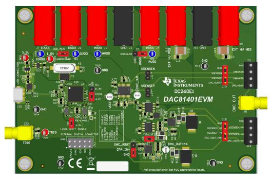
Figure 3-2. Default Header Settings with High Voltage Gain Stage Disabled
