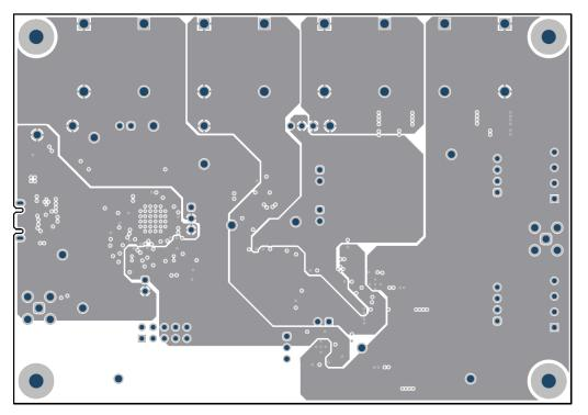
Figure 4-6. DAC81401EVM PCB Mid Layer 1 Layout
