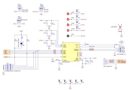
Figure 4-2. DAC81401EVM Schematic : DAC81401 Interface
