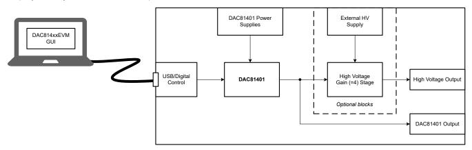
Figure 3-3. DAC81401EVM Hardware Setup
