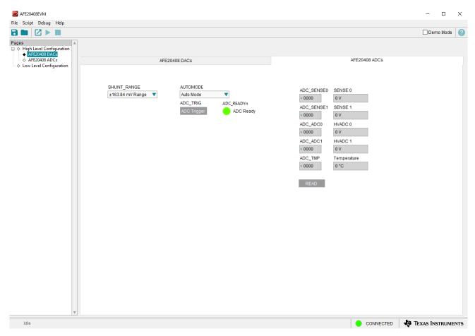
Figure 3-8. ADC Control Tab of the High Level Configuration Page
