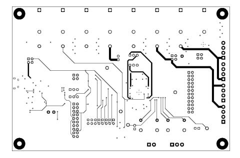
Figure 4-7. AFE20408EVM PCB Bottom Layer Layout
