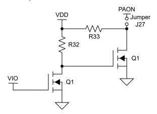
Figure 2-4. AFE20408EVM PAON Open Drain Circuit
