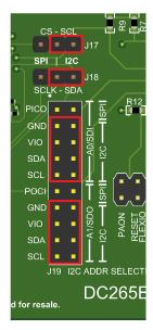
Figure 2-3. AFE20408EVM Configuration I<sup>2</sup>C
