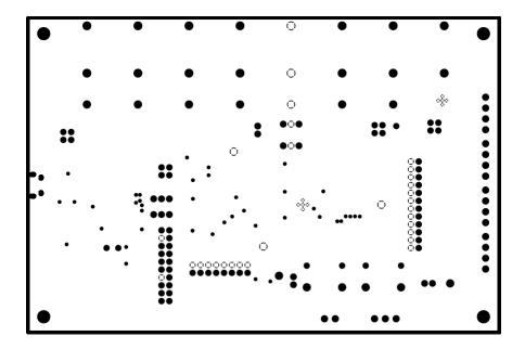
Figure 4-5. AFE20408EVM PCB Mid Layer 1 Layout (Ground Plane)
