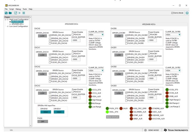
Figure 3-7. DAC Control Tab of the High Level Configuration Page
