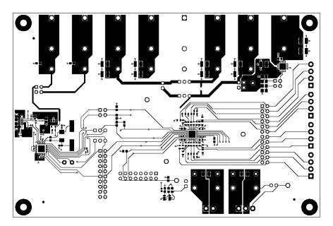
Figure 4-4. AFE20408EVM PCB Top Layer Layout
