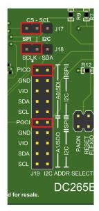
Figure 2-2. AFE20408EVM Configuration for SPI
