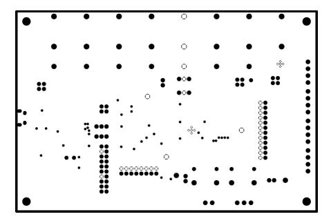
Figure 4-6. AFE20408EVM PCB Mid Layer 2 Layout (Ground Plane)
