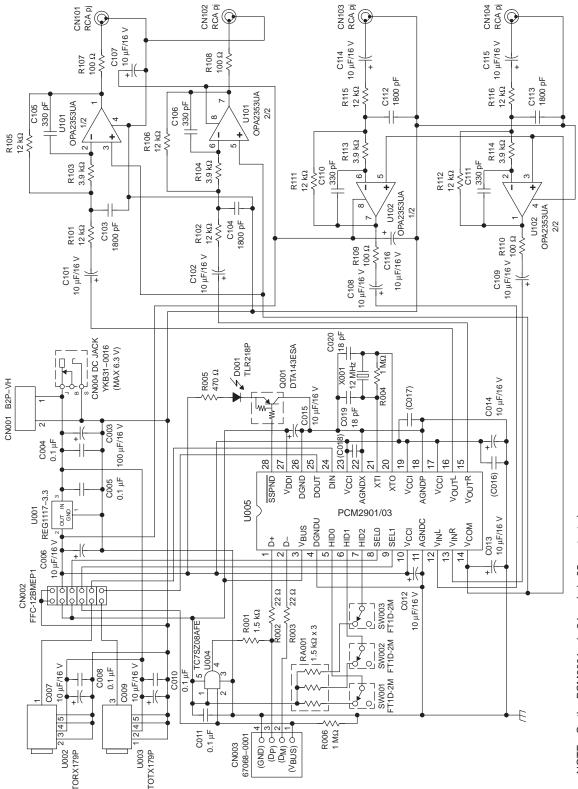
NOTE: On the PCM2901, pin 24 and pin 25 are test pins.
