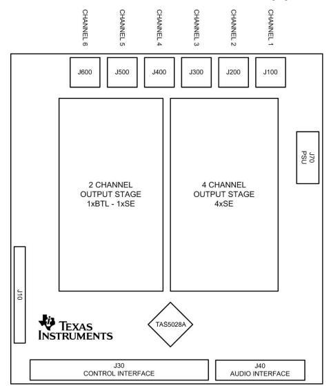
Figure 1-2. Physical Structure for the TAS5028-5122C6EVM (rough outline)
