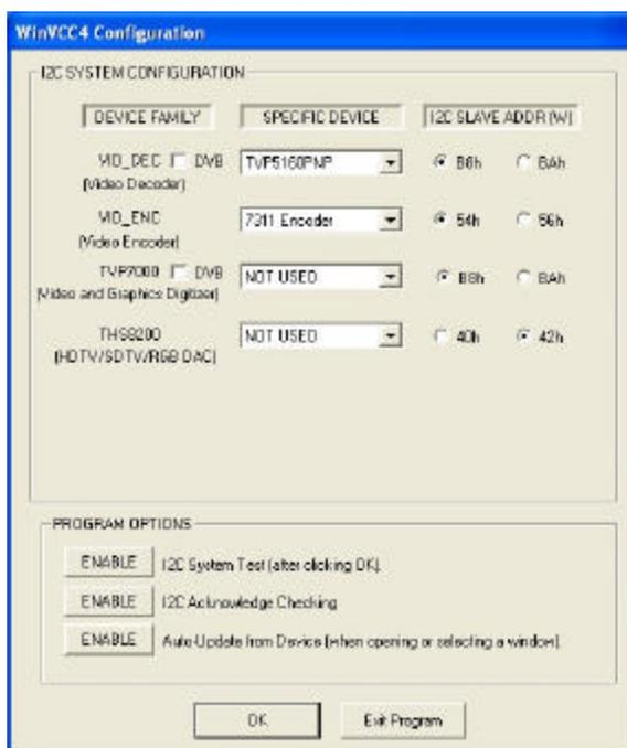
**Figure 1. WinVCC4 – I<sup>2</sup>C Configuration Screen**
