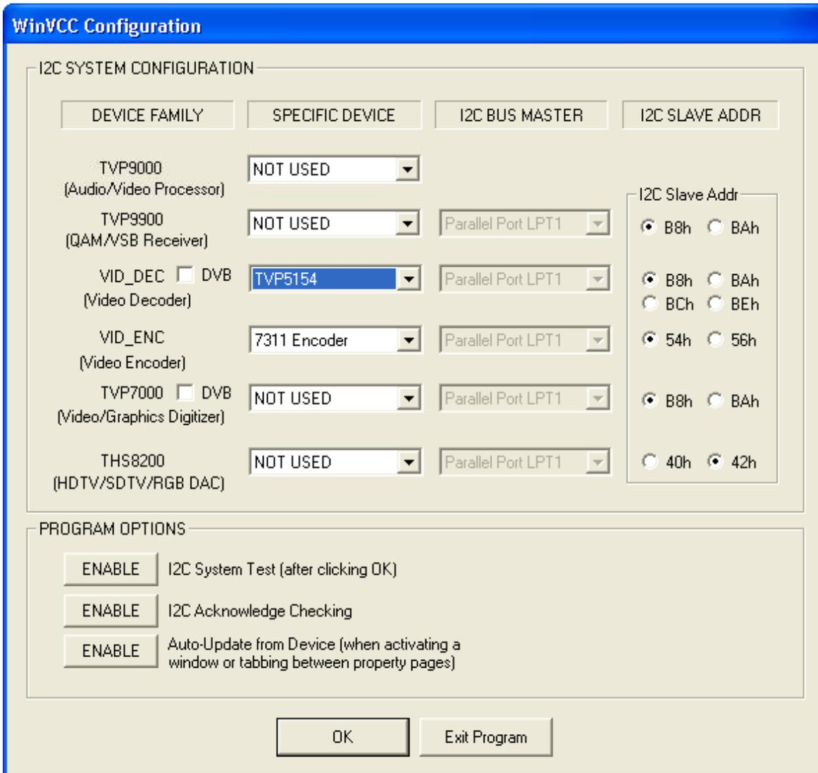
**Figure 1. WinVCC – I<sup>2</sup>C Configuration Screen**
