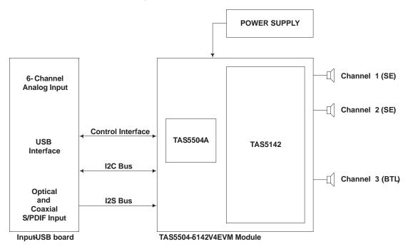
Figure 4-1. Integrated PurePath Digital™ Amplifier 2.1 System
