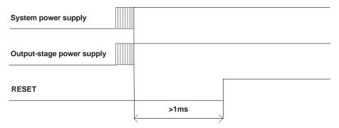
Figure 2-1. Recommended Power-Up Sequence
