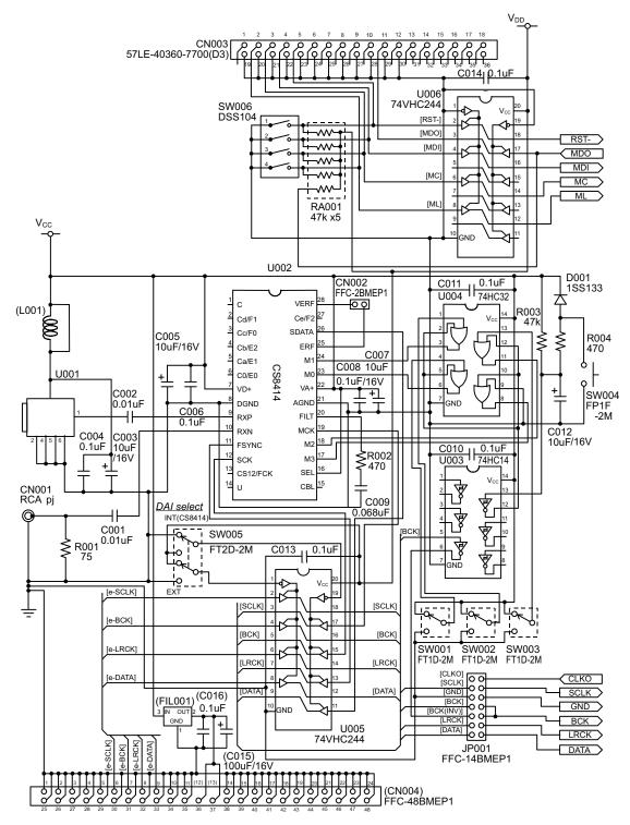
Figure 4. DEM-DAI/DAC Digital Audio Interface
