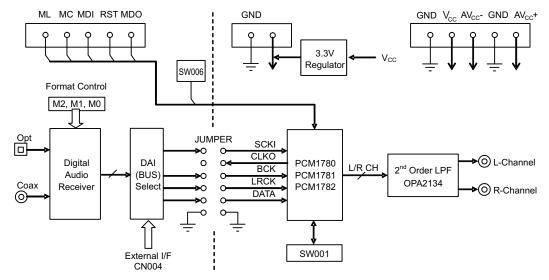
Figure 1. DEM-DAI1780/1781/1782 Block Diagram
