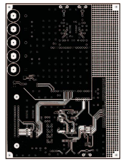
Figure 7. DEM-DAI/DAC Top View
