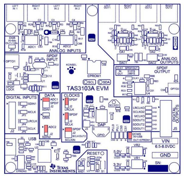
Figure 2-3. Enable Analog Input Configuration
