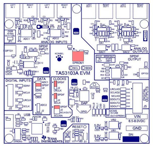
Figure 2-2. Load Configuration Data From EEPROM
