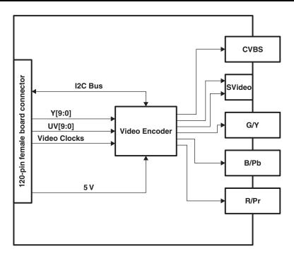
Figure 1-2. Encoder Module
