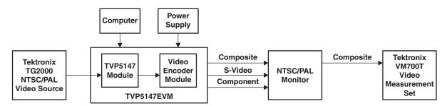
Figure 1-5. TVP5147EVM System Level Block Diagram
