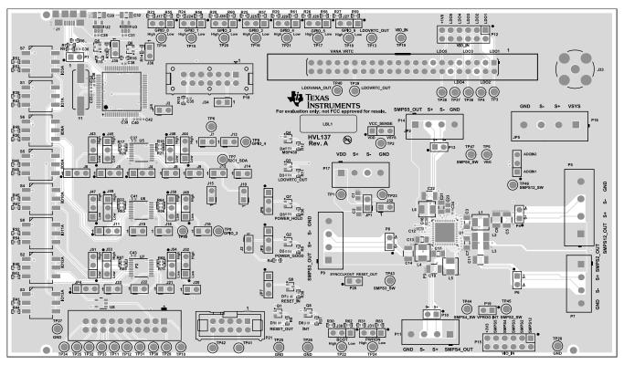
Figure 7. Composite - Top View
