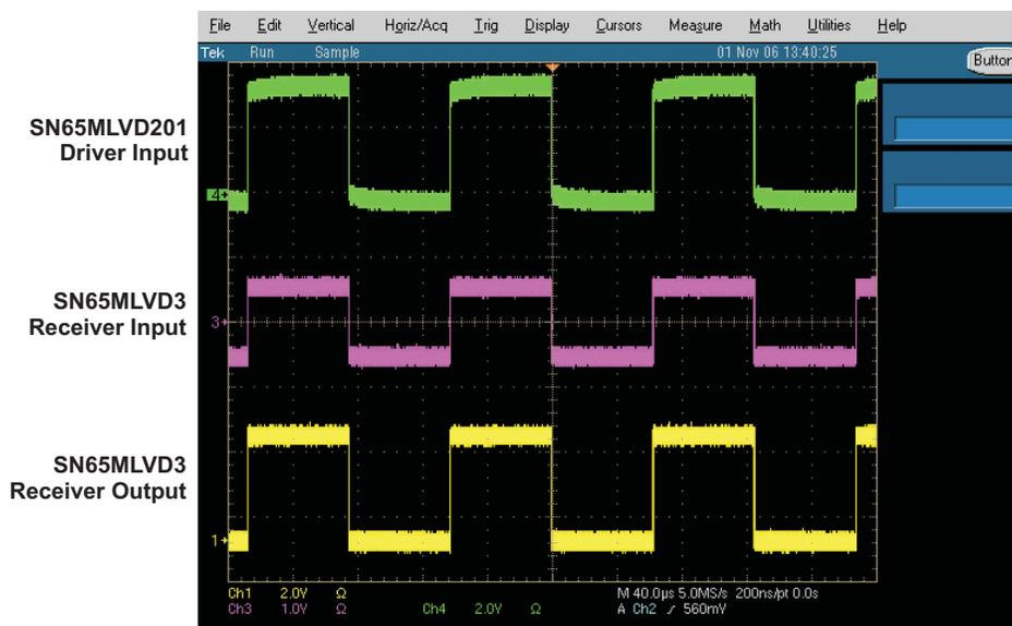
**Figure 15. Parallel Terminated Point-to-Point Parallel Simplex Typical Eye Pattern at 8 kHz with High-Impedance Output Termination**
