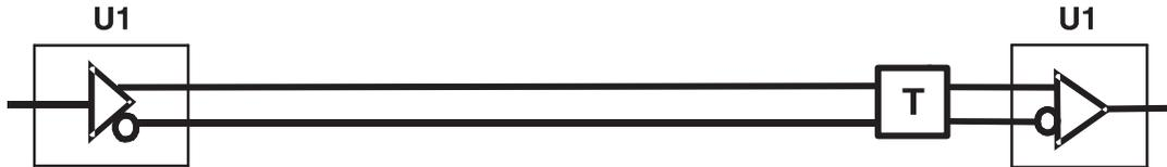
**Figure 3. Point-to-Point Simplex Circuit**
