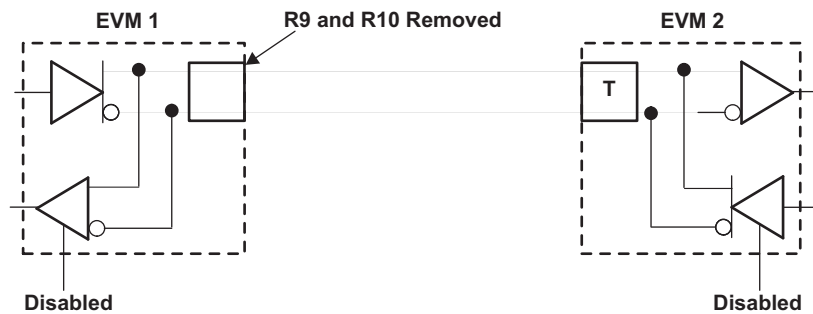
Figure 5. Point-to-Point Simplex Circuit
