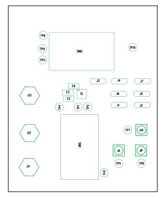
Figure 3. Assembly Top Layer
