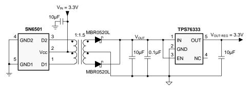
Figure 1, SN6501-3EVM Pinout and Functional Block Diagram
