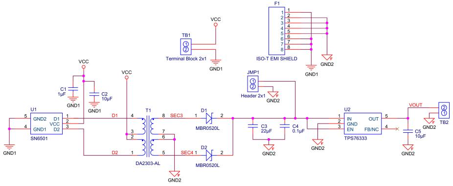
Figure 2. SN6501-3EVM Schematic
