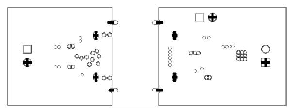
Figure 5. SN6501-3EVM Ground Plane View
