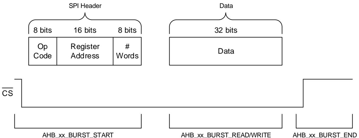
[Figure 12](#) shows how a single word read or write can be broken up into 3 functions. The START function pulls CS low and sends the SPI header. The READ/WRITE function is responsible for reading or writing a single word at a time, for however many words were stated in the SPI header. The END function is responsible for pulling the CS high, to signal the end of the transfer.
