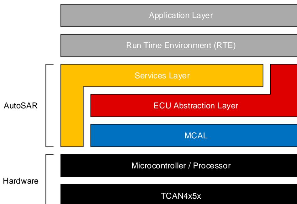
Texas Instruments provides the necessary ECU abstraction layer driver source code necessary to integrate the TCAN4550-Q1 into an AutoSAR environment. Contact TI to get the source code.
