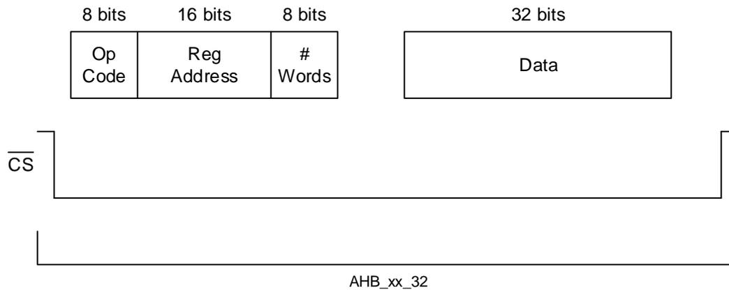
In [Figure 11](#), a single 32-bit ( 1 word ) SPI read or write example is shown. The first word contains the SPI header, which tells the TCAN4550-Q1 what action to perform (read or write), what register address to start at, and how many words of data to read/write.
