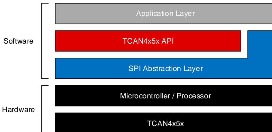
This Microcontroller Abstraction source code is developed for a MSP430FR6989 and is functional with the MSP-EXP430FR6989 LaunchPad. The code can be used with other microcontrollers and processors by updating the appropriate SPI drivers.
