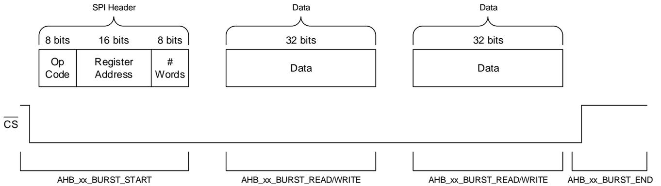
Figure 13 shows a 2 word SPI transfer example, and how the READ/WRITE function is called twice to do each individual word transfer. This is helpful for cutting down on the SPI overhead when transferring a CAN message to or from the TCAN4550-Q1, and minimize the maximum SPI frequency required.
