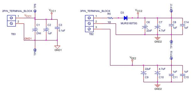
Figure 1. ISO5851 EVM Power Supply Schematic
