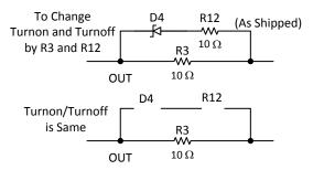
Figure 9. To have different Turn-on and Turn-off
