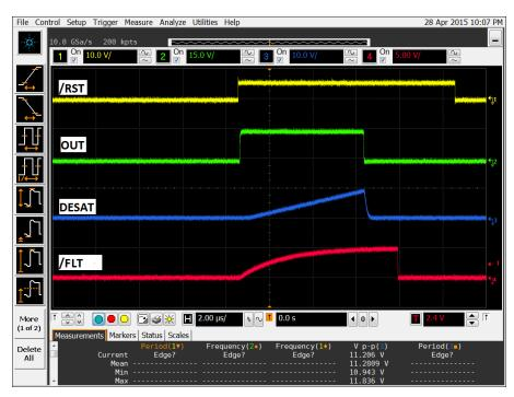
Figure 7. ISO5851 EVM DESAT and Reset with Bipolar Output Supply
