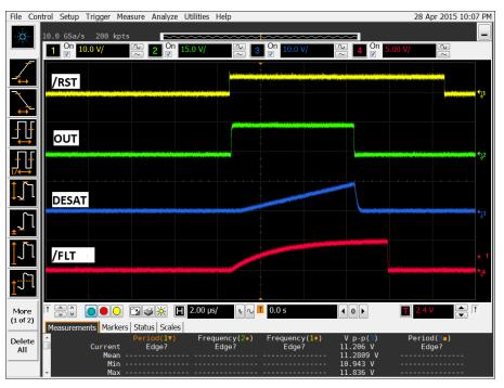
Figure 6. ISO5851 EVM DESAT and Reset with Unipolar Output Supply
