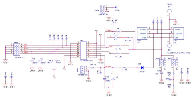
Figure 3. ISO5851 EVM Signal Path Schematic
