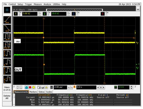
Figure 5. ISO5851 EVM Input and Output With Bipolar Output Supply (V<sub>cc2</sub> = 15-V, V<sub>EE2</sub> = -8-V)
