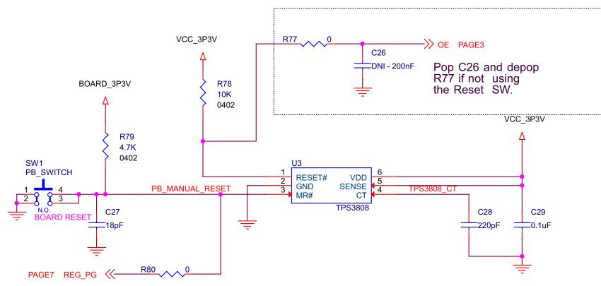
Figure 9. DP149RSBEVM Reset Schematic
