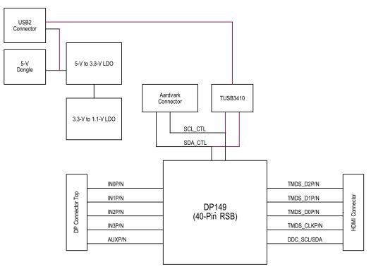
100- $\Omega$  differential impedance for HDMI differential pairs.
