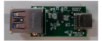
Figure 2. HD3SS3220 UFP Dongle
