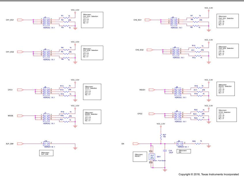
Figure 4. TUSB522P EVM Schematic (Device Control Pins)
