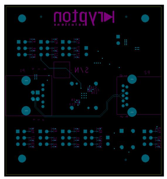
Figure 8. EVM Layout Layer 4 (Bottom)
