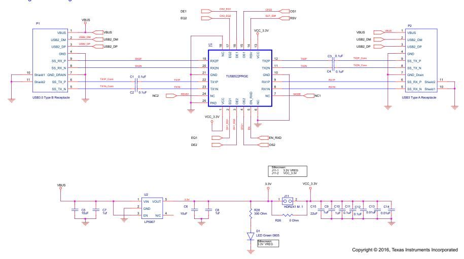
Figure 3. TUSB522P EVM Schematic (High Speed Pins / Power)
