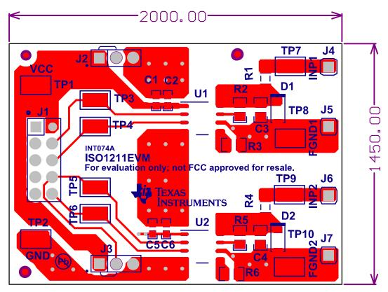
Figure 8. ISO1211EVM PCB Layout—Top Layer
