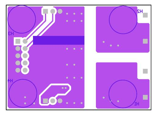
Figure 9. ISO1211EVM PCB Layout—Bottom Layer
