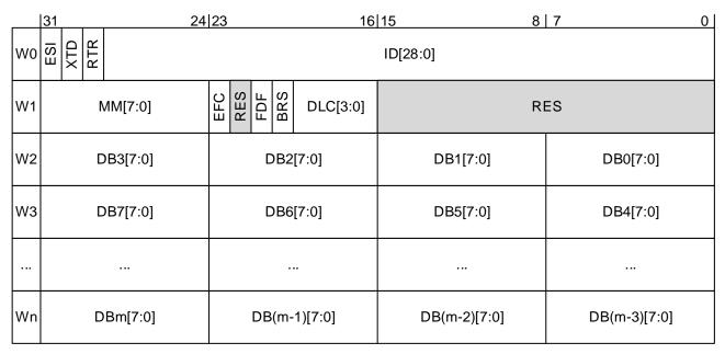
Figure 12. Tx FIFO / Buffer Element
