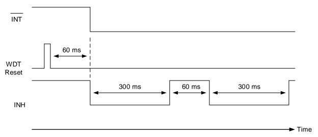
Figure 4. Example Watchdog Timer Behavior (60 ms and INH output)
