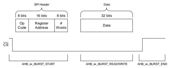
Figure 20. SPI Packet Breakdown
