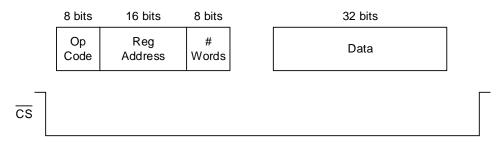
Figure 19. 32-bit SPI Read or Write Example
