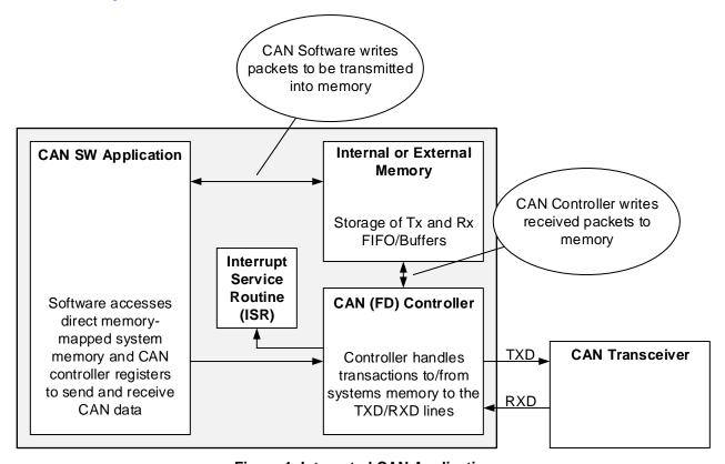
Figure 1. Integrated CAN Application
