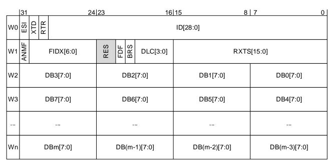
Figure 10. Rx FIFO / Buffer Element
