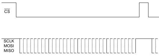
Figure 14. An Example Efficient SPI Transfer
