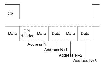
Figure 16. Efficient Transfer of Large Data
