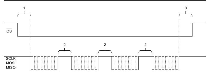
Figure 13. An Example Inefficient SPI Transfer
