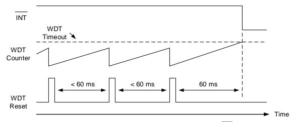
Figure 3. Example Watchdog Timer Behavior (60 ms and INT output)
