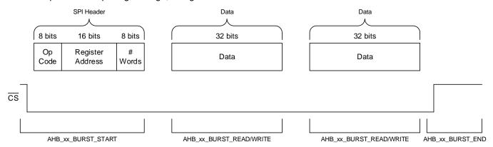
Figure 21. Multi-word SPI Packet Example
