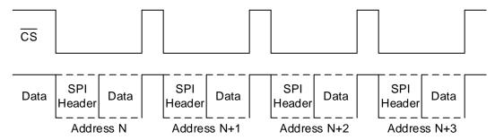
Figure 15. Inefficient Transfer of Large Data
